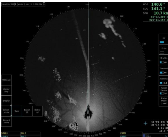
(b) Ice-breaker radar track shows the route it took through the ice.
